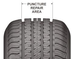
**NOTE:** Puncture repairs should be confined to the tread area only as shown. The repair must be referred to a full-service repair facility<sup>1</sup> if the injury is larger than 1/4" or if the injury(ies) are located in the sidewall or bead areas.
